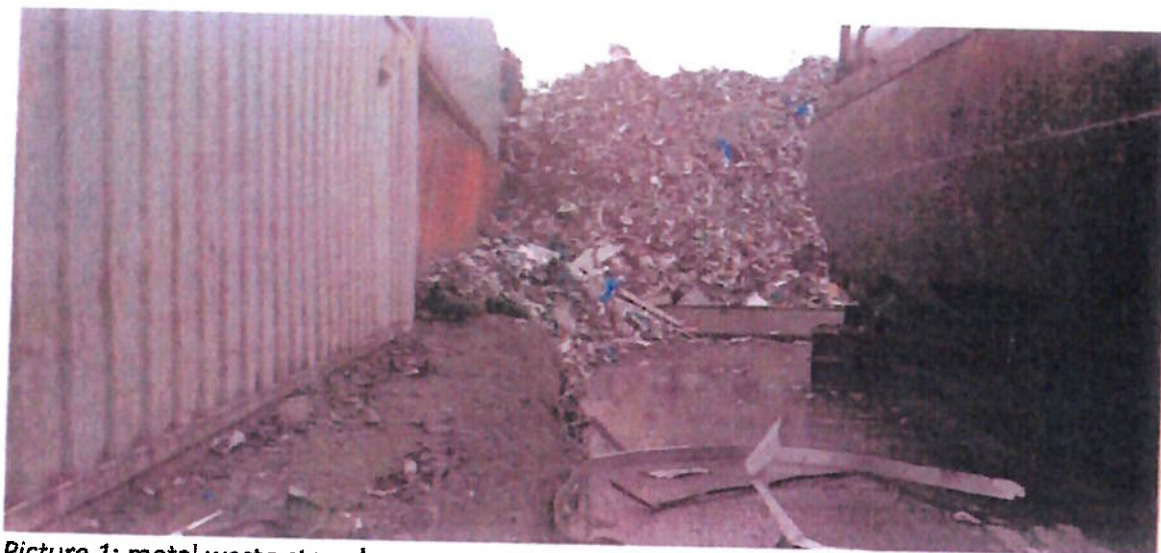
Picture 1: metal waste stored on a non concrete surface in southwestern corner.
